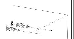
Tap anchors [C] into pilot holes. Hand tighten with #2 Phillips screwdriver (Use in drywall only.)
