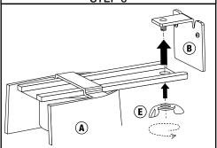
Secure main unit [A] to wall bracket [B] with wing nut [E]. Do not overtighten. Installation is complete.
