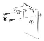
Align bracket [B] and attach with screws [D] (or use hardware suitable for your backsplash material).
