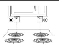
Align wall bracket [B] with center line of burners.
