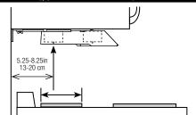
The center of the rear canister must be over the rear burner. If not, go to www.STFS.com to order an extension bracket kit.
